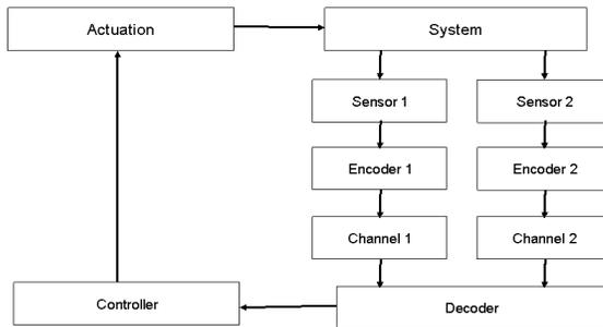
Fig. 4. The structure of our optimal LQG control solution for the two-sensor case (Case  $C_2$ ).
