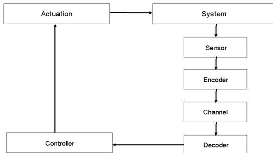
Fig. 3. The structure of our optimal LQG control solution (Case  $C_1$ ).
