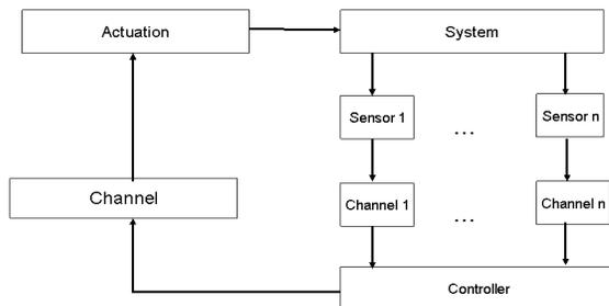
Fig. 1. The architecture of a packet-based control loop. The channels are unreliable and unpredictably drop packets.
